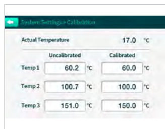
Accurate temperature control with 3-point calibration
