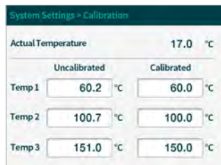
Accurate temperature control with 3-point calibration
