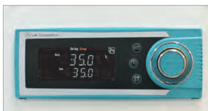
General controller with clear VFD panel (OF3)
