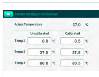
Accurate temperature control with 3-point calibration
